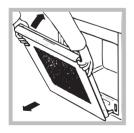
3. Grip the door on the two outer sides and close it approximately half way. Pull the door towards you, lifting it out of its slot (*see diagram*). To replace the door, reverse this sequence.
